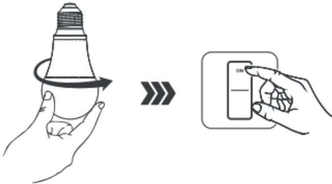
Install the light bulb (screw it in clockwise) and connect the ignition switch.
